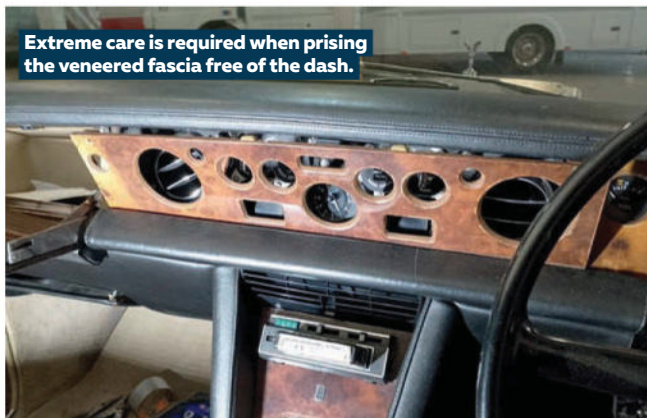
At last! Dash roll removal represents lots of effort to get at two small wooden strips.
