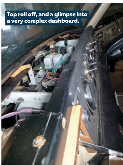
Tiny, soft screws held the dash-top strip in place.
